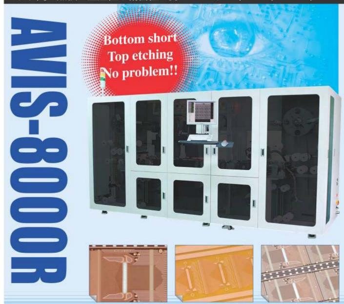
AVIS-8000R is an Automatic Vision Inspection System for both of pattern defects (AOI) and SR defects (AFVI) on COF/TAB, TBGA, H2BGA, FBGA with highest inspection productivity and accuracy.
